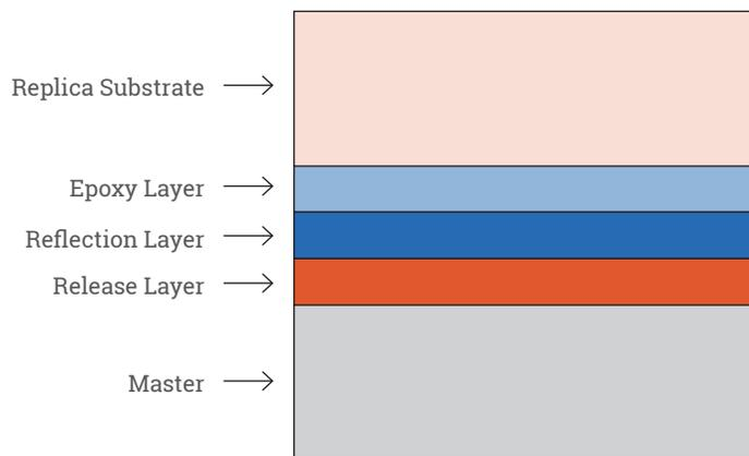
3. Once the epoxy has cured, the replica is separated from the master with the epoxy and reflective coating intact. The surface properties of the master have now been transferred to the substrate.
